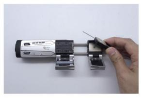
2. Open the both covers and put the holder with fiber on the right slide.
