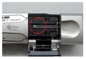
4. Slide the fiber holder with cover closed into the thermal stripper.
